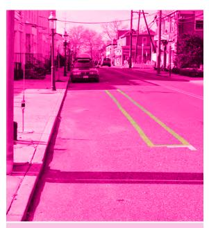
Striping applied inside of the parking lane in Cape May, New Jersey, makes "No Parking" zones more visually apparent both to drivers looking for a spot and to parking enforcement officials.
