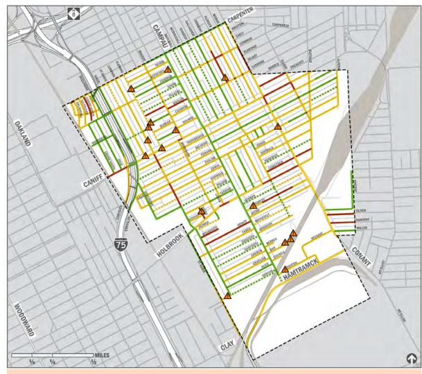
Detailed Street Condition. Dotted Lines indicate recently repaired street surfaces. Source: Interface Studio.
